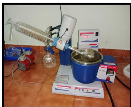
Figure 02: Rotary vacuum evaporator.
