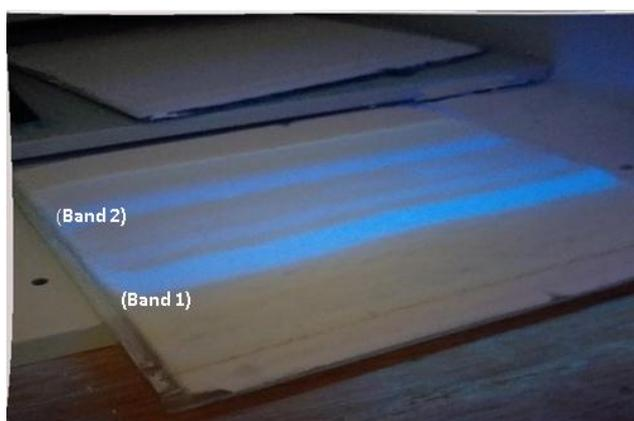
Figure 1: Bands of TLC silica gel plate under UV lamp (366 nm).
