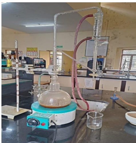
Fig.5.3: Extraction of clove oil from clove using Clevenger apparatus.
