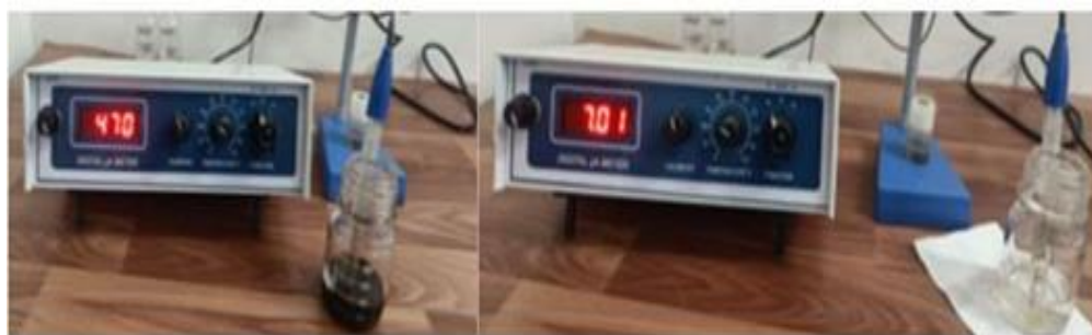
Fig. 5a: OP pH at first and last wash.
