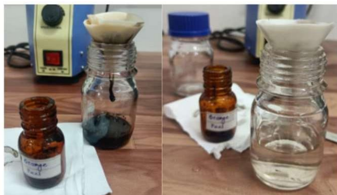
Fig. 4a: Rinsing OP 1 st wash and last 5 th wash.
