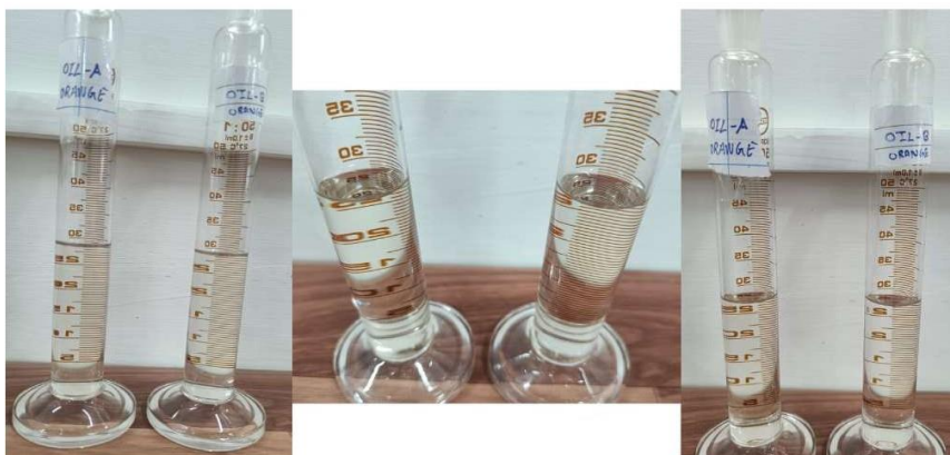
Fig. 11 a: In oil sample 'A' and 'B' prepared using orange peel complete transparent clear solution obtained.
