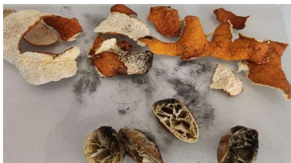
Fig. 1: OP and LP dried at 80 °C for 36 hours to get brittle.
