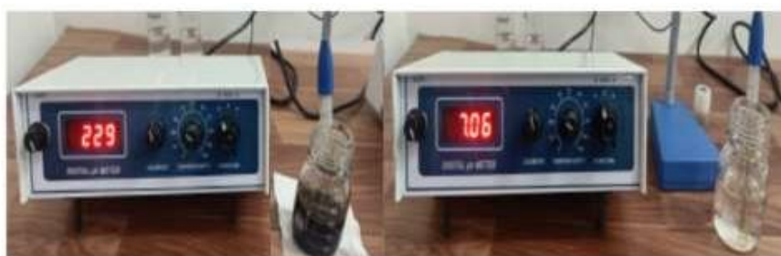
Fig. 5b: LP pH at first and last wash.
