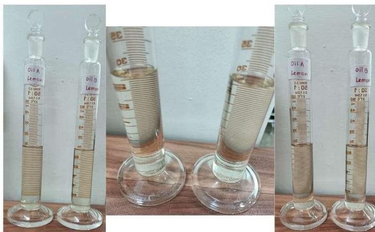
Fig. 11 b: In oil sample 'A' and 'B' prepared using lemon peel with no turbidity at the bottom of measuring cylinder obtained.
