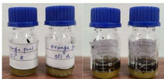
Fig. 7: A very thin upper layer was observed, along with a thick lower layer of petroleum jelly. (OP Front View and Back View).
