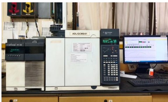
Figure 9: Agilent Technologies 5977A-MSD GC-MS system used for phytochemical profiling.
