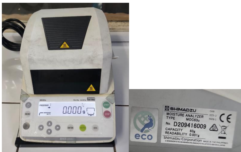
Figure 12: Moisture Analyzer Shimadzu (Model MOC63u) used for moisture content determination.
