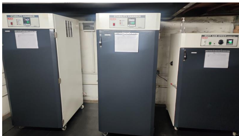
Figure 15: Labline Hot Air Oven (Model LSC-351) used for moisture content determination and Labline Stability Chamber (Model LSC-320) used for stability studies.
