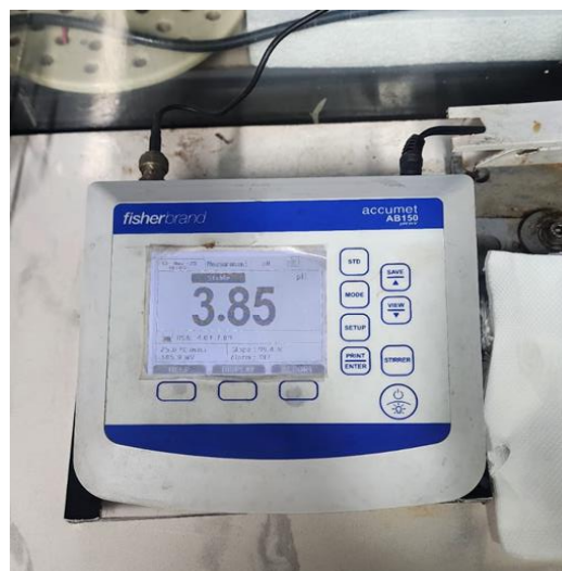
Figure 11: Fisher Brand Accumet AB150 pH meter used for pH determination.
