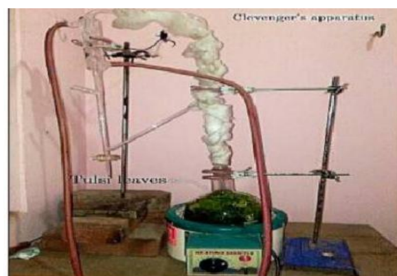
Figure 1: Actual image of the apparatus used during the extraction of tulsi oil.
