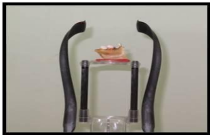
Figure 1 Mounting of bone specimen on a jig for obtaining CBCT scan.
