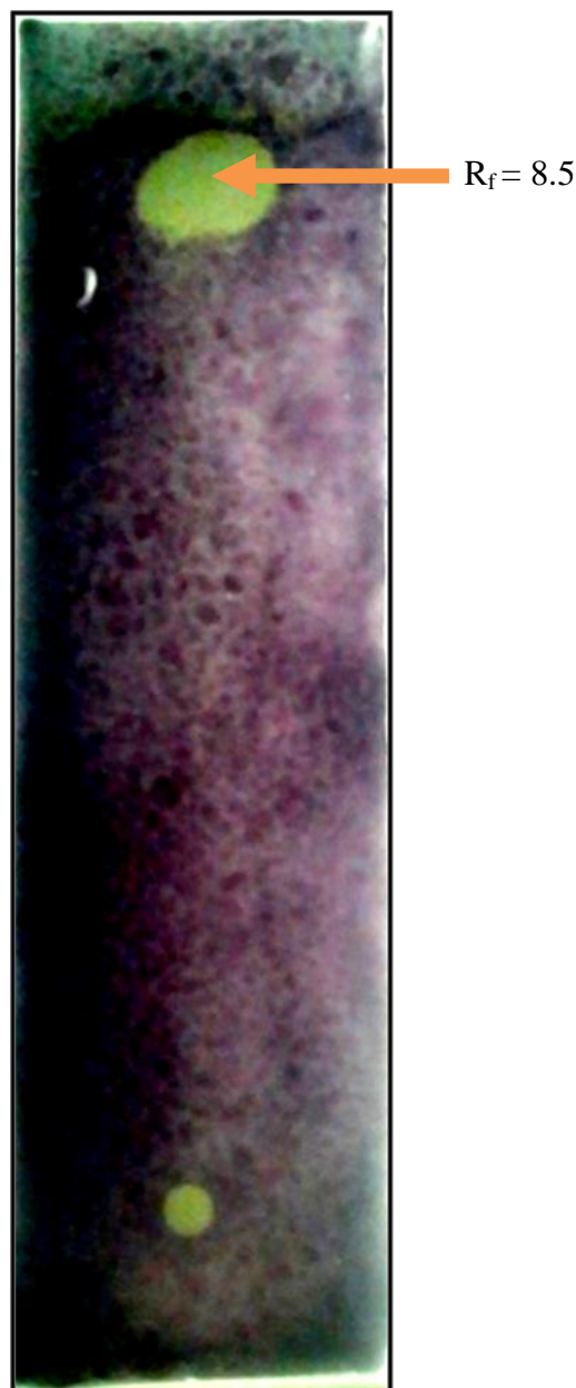
Fig 3: Thin layer chromatograph of potent antioxidant fraction obtained from gel filtration chromatography. The material around the R_f value of 8.5 was scratched off and sent for LC MS analysis.
