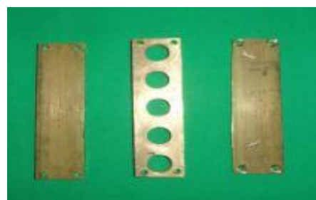
FIGURE 5 : Standardized 3 piece brass mould for hardness specimen
