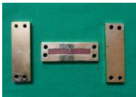
FIGURE 6 : After curing brass mould with heat cure blocks were opened.
