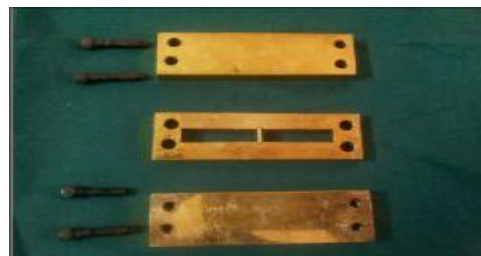
FIGURE 4: Standardized 3 piece brass mould for tensile strength specimen
