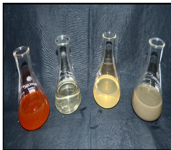
(A) (B) (C) (D) A- Plant Extract B- Only Silver Nitrate solution C- Initial Stage of Silver Nanoparticles Synthesis D- Synthesis of Silver Nanoparticles
