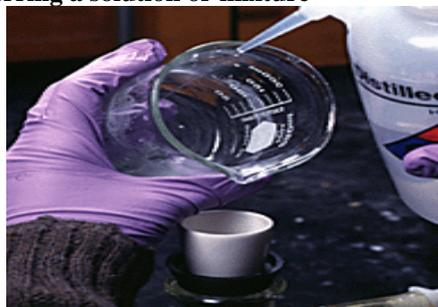
If you are transferring a solution or heterogeneous mixture to another vessel, rinse the container with solvent to be sure the transfer is quantitative. The rinsing should be transferred to the second vessel along with the rest of the mixture or solution.
