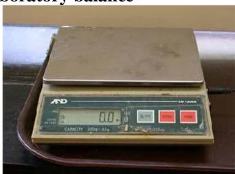
A standard laboratory balance is used for preparative work where an error of  $\pm 0.02$  g is acceptable. It is also often used for pre-weighing samples to determine the mass approximately. The exact mass is then determined using an analytical balance.
