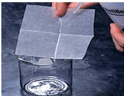
Finally, the paper should be rinsed into the beaker, to remove all traces of the solid.
