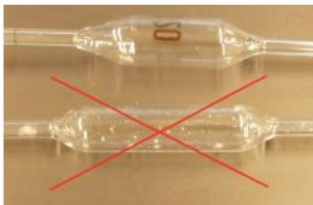
**Fig. 2:** a clean and a badly contaminated 20 ml transfer pipette
