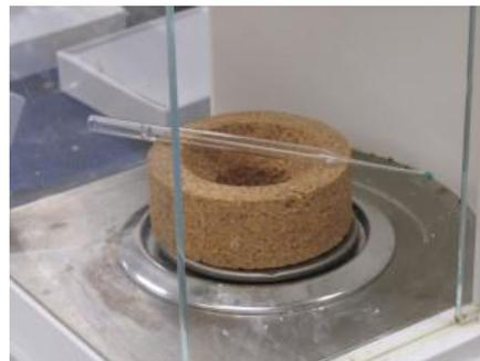
Weighing via pipette: Measuring marker ink in acetone, for visibility.
