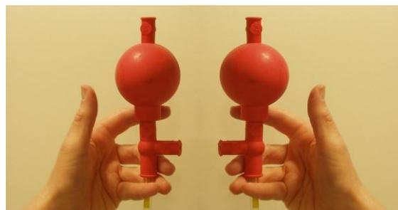
**Fig. 4:** left-handed and right-handed grip of the filler and pipette
