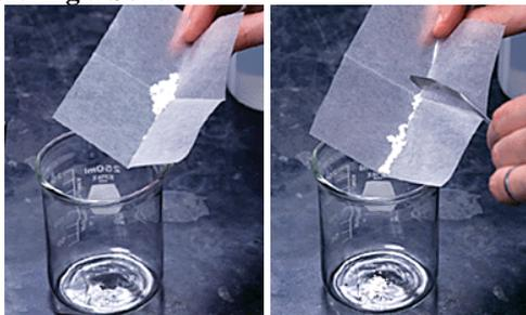
This can be done by carefully tipping the creased weighing paper to pour the solid into the beaker. Tapping the paper with a spatula will knock particles into the beaker.
