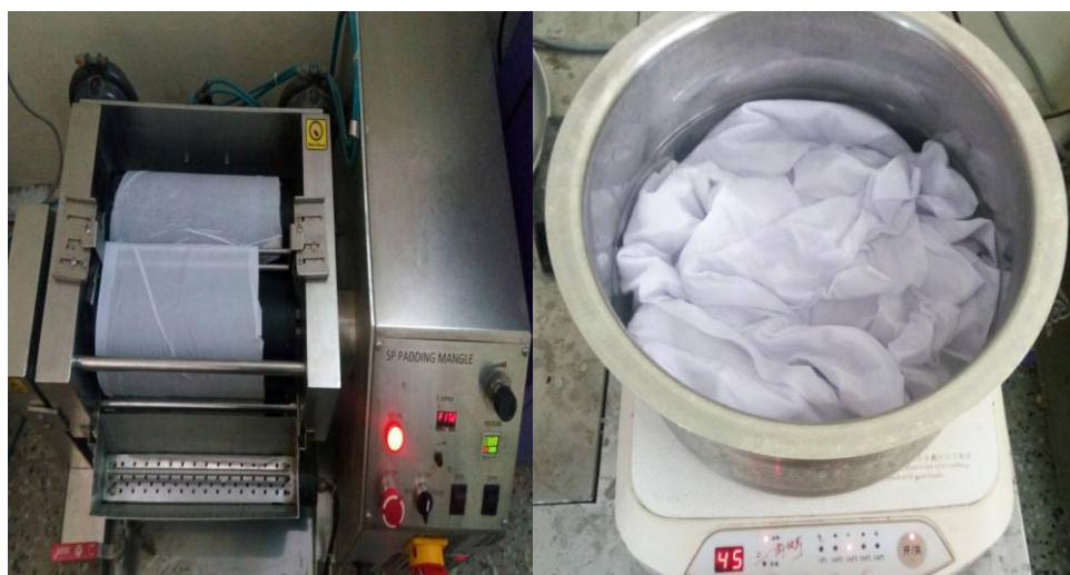
Figure 2: Pad-dry and dip-dry method.
