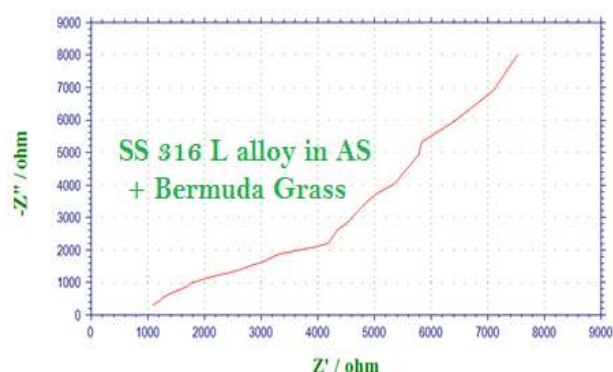
Fig. 3: Nyquist plot of SS 316 L alloy immersed in AS + Bermuda grass extract.
