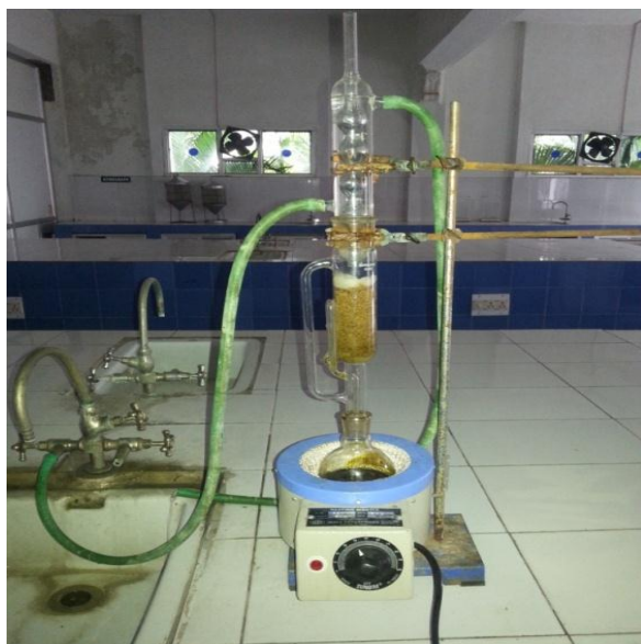
Plant extraction through soxlet apparatus
