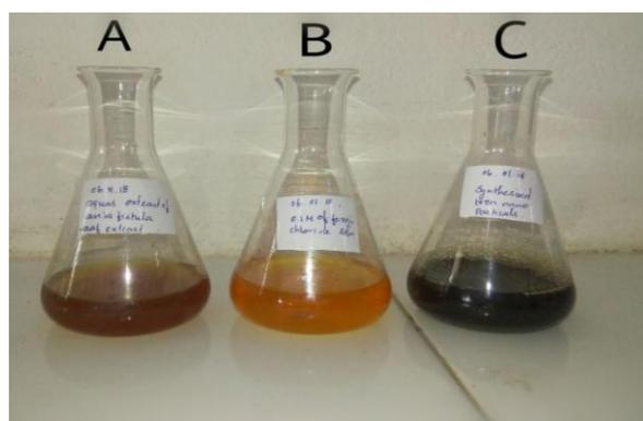
**Figure 1: Change in color from brown to black indicates the synthesis of Iron Nanoparticles.**
