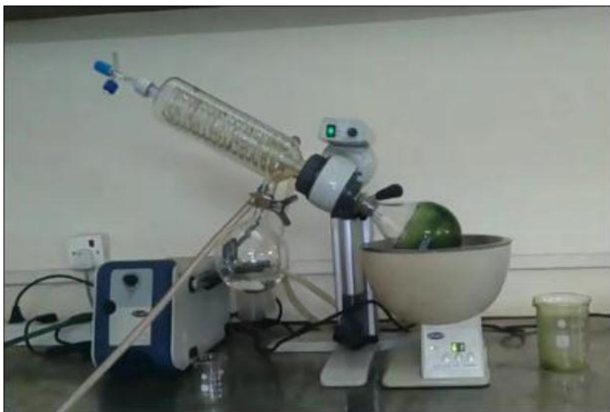
Fig1: Evaporation of the solvent with rotary evaporator.
