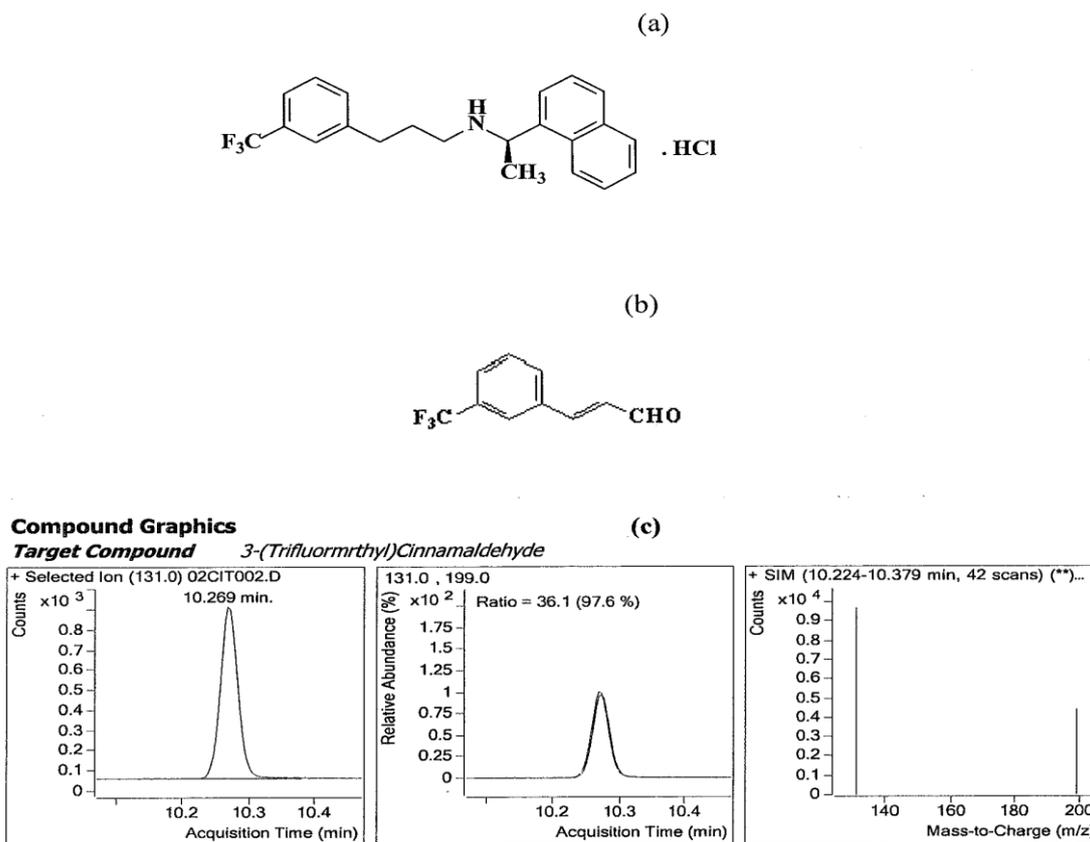
**Fig. 1. The structures of (a) Cinacalcet hydrochloride, (b) 3-(Trifluoromethyl) cinnamaldehyde and (c) Mass spectrum of 3-(Trifluoromethyl) cinnamaldehyde**
