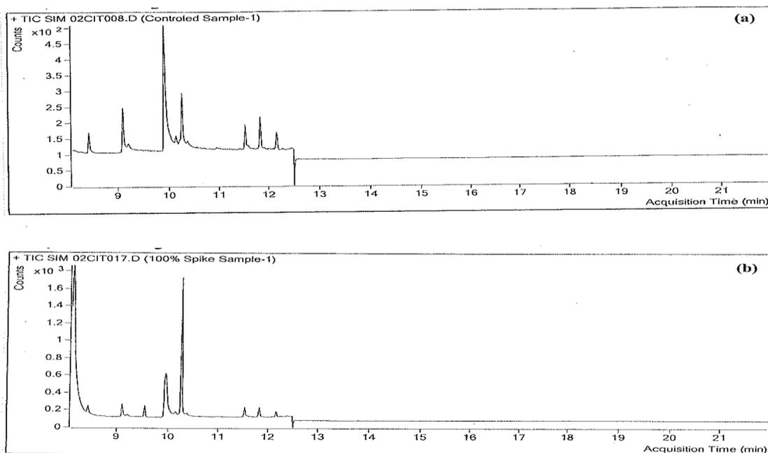
Fig. 2. Typical representative overlaid chromatograms of (a) Control sample and (b) Spiked sample
