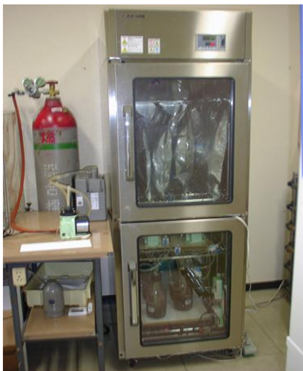
Figure 1: Experimental incubation chamber with the four reactors systems.
