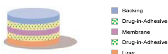
Fig. 3 Multi laminate type
