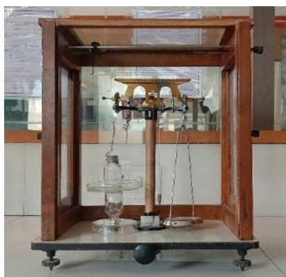
Fig 2: Modified Mucoadhesive Strength Apparatus.
