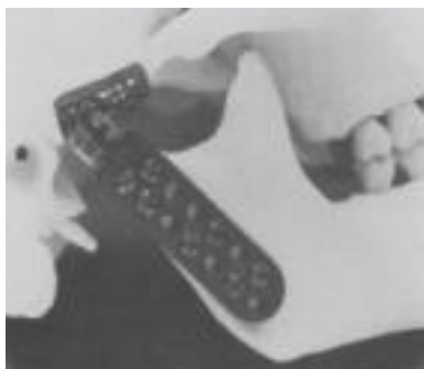
Fig. 8: Patient-Specific all metal TJR mounted on a stereolithography model of the patient for which the prosthesis was fabricated.
