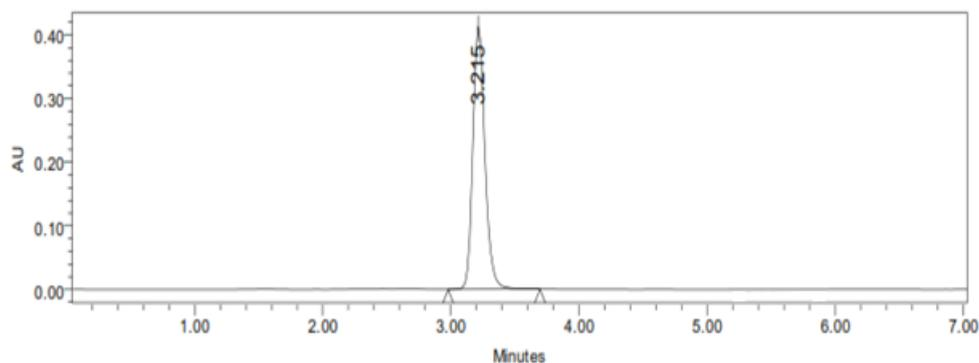
Fig-3: Optimized Chromatographic Condition of Linagliptin.
