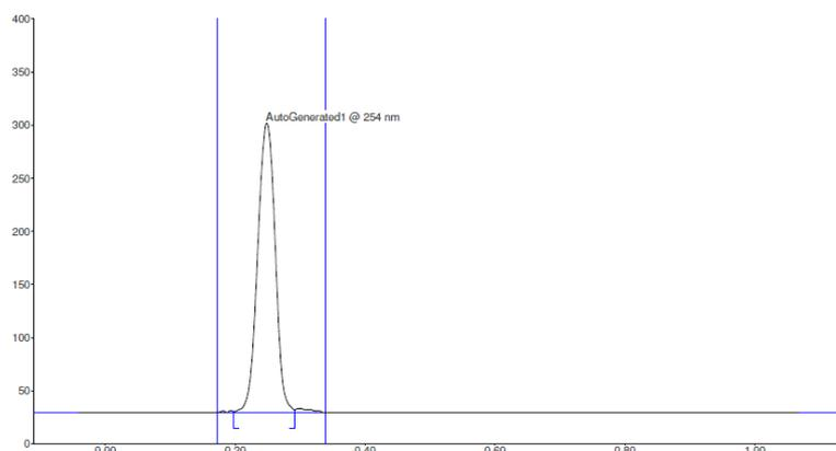
Figure 3: Densitogram of standard valacyclovir hydrochloride; ( $R_f$ :  $0.22 \pm 0.01$ ), mobile phase n-butanol: methanol: Water (3:1:1 v/v/v).
