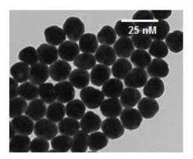
**3.3 SEM** SEM images provided information about the morphology and size of the biosynthesized silver nanoparticles. The silver nanoparcticles were found to be spherical in shape. The diameter of synthesized silver
