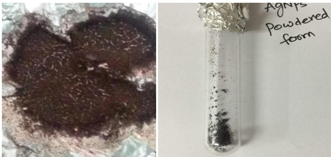
Fig-6&7: showing sun dried Pellet and powdered form AgNPs
