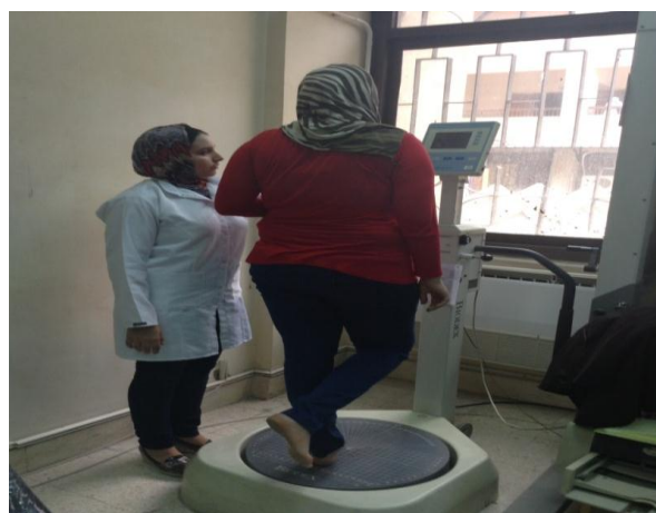
(Figure.16) Application of biodex balance system (dynamic stability test). Faculty of physical therapy, Cairo University.
