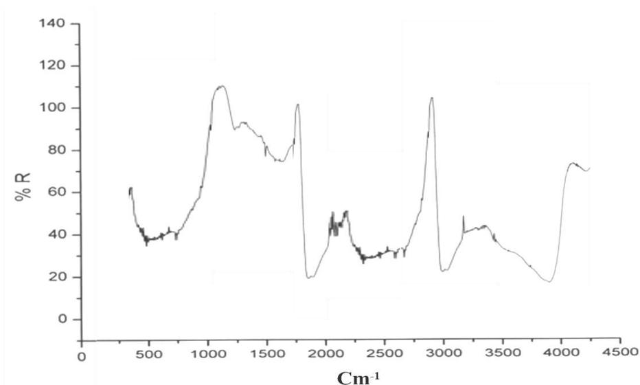
Fig. 2: FTIR spectrum of copper nanoparticles.
