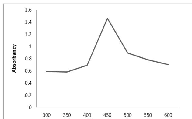
Fig. 1: UV-Vis spectrum of copper nanoparticles.
