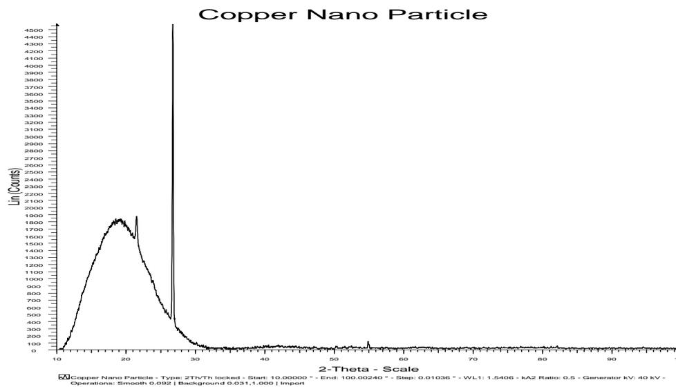
Fig. 3: XRD analysis of copper nanoparticles.
