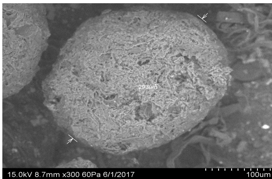
Fig 2 Scanning electron microscopy of a) surface morphology of drug-loaded microspheres by ionic gelation method, b) surface morphology of drug loaded microsphere by emulsion- ionic gelation method.
