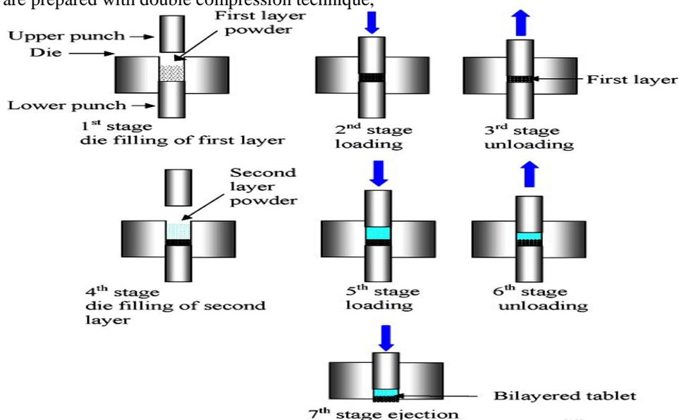
Fig. 11: Steps Involved In Preparation of Bilayer Tablets.<sup>[13]</sup>
