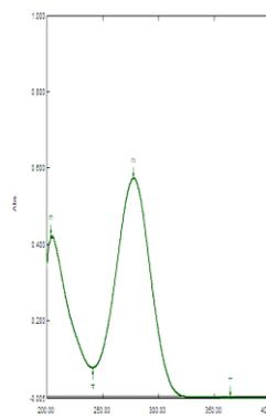
**Figure-7: UV Maximum Absorbance  $\lambda_{\text{max}}$  of Sultamicillin.**
