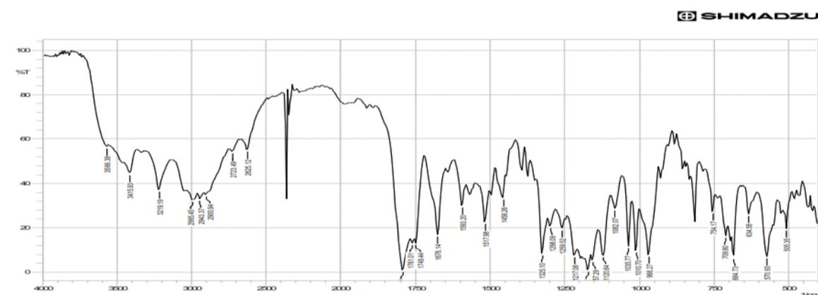
**Figure-6: Infra Red spectra of Sultamicillin tosilate (Standard & API).**
