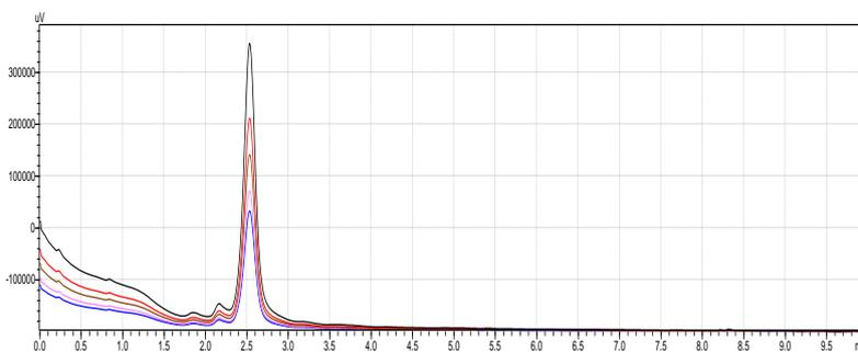
**Figure-13: Overlain Linearity Chromatogram of Sultamicillin.**
