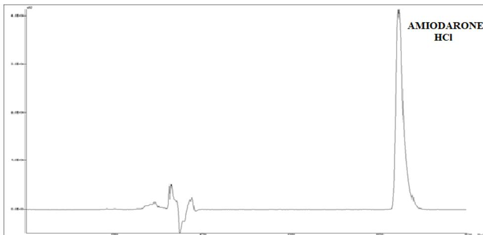
**Fig. 8: Chromatogram of Amiodarone hydrochloride after UV light exposure.**
