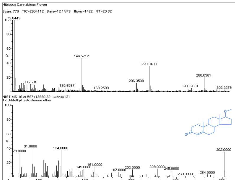
**Fig. 7: Mass spectrum of 17-O-methyl testosterone ether.**
