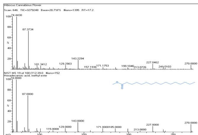
Fig. 3: Mass spectrum of Hexadecanoic acid, methyl ester.
