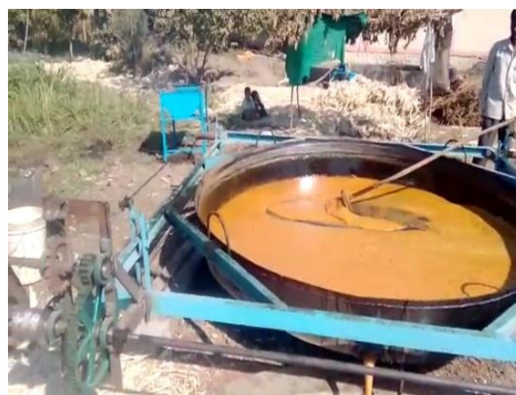
Fig. 3: Open pan mounted on power mechanism lifter and drain into cooling pit.
