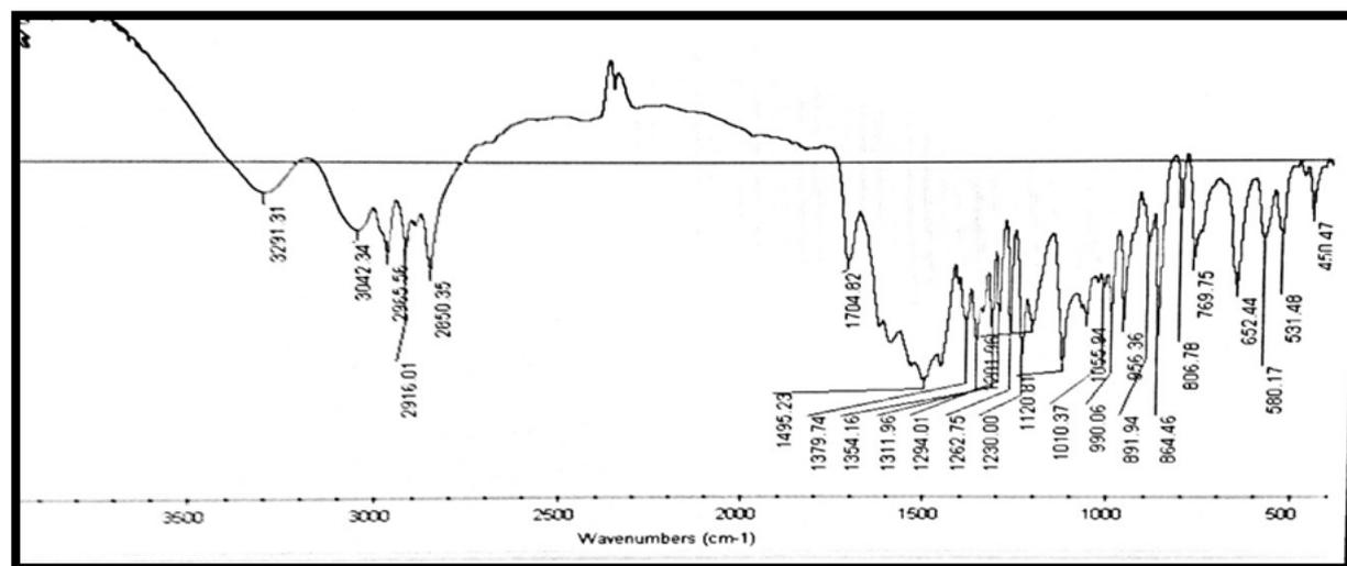
**Figure 3: FTIR of Timolol Maleate with Croscarmellose Sodium.**
