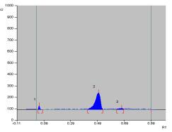
Fig. 6: HPTLC densitogram of Sorafenib tosylate in acidic stress condition.
