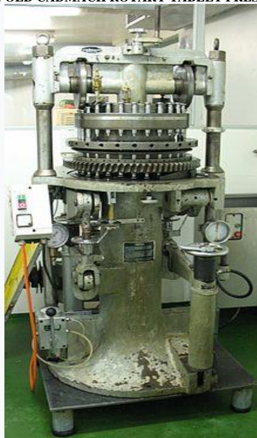
Figure 13: Cadmach Rotary Tablet Press.
