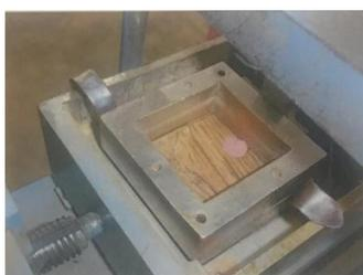
**Figure 3: Split shear bond testing.**
