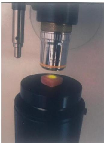
**Figure 2: Vicker's Hardness Test.**
