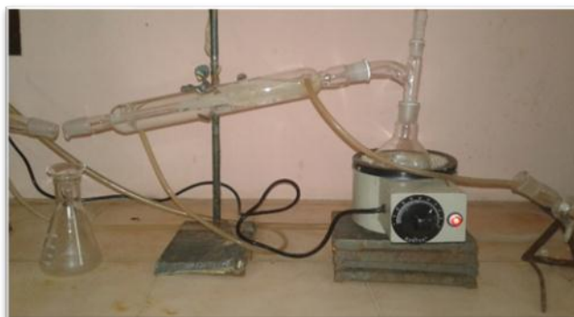
Fig. 1: Simple distillation process setup.
