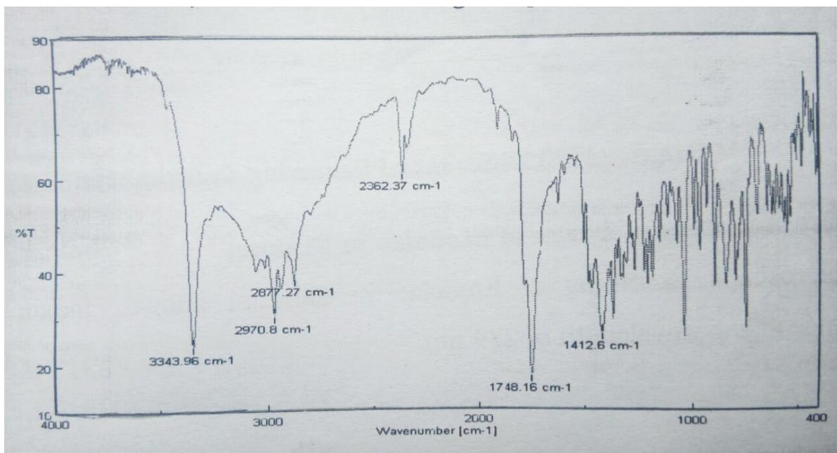
**Fig. 6: Fourier transform infrared spectrum of copper nanoparticles.**
