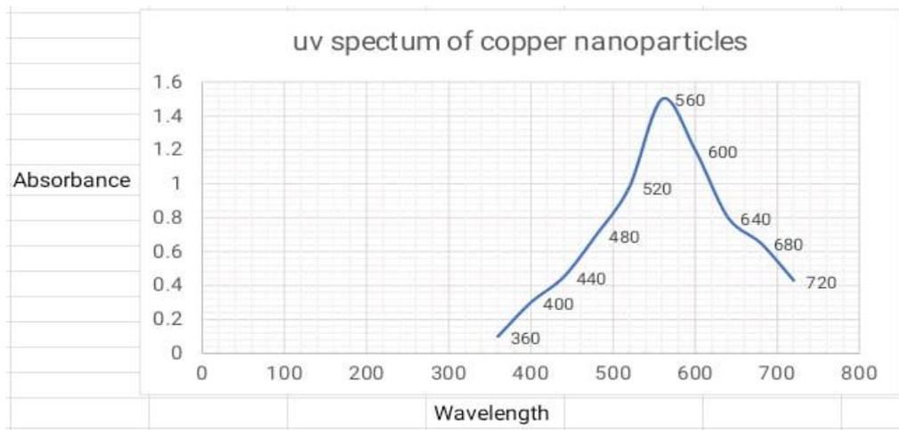
**Fig. 5: UV Visible spectrum of copper nanoparticles.**
