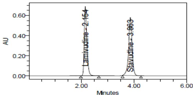
Figure 4: Chromatogram of accuracy 150% solution
