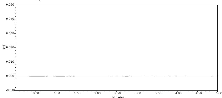
**Figure 10: Chromatogram for checking baseline noise of LOD solution.**
