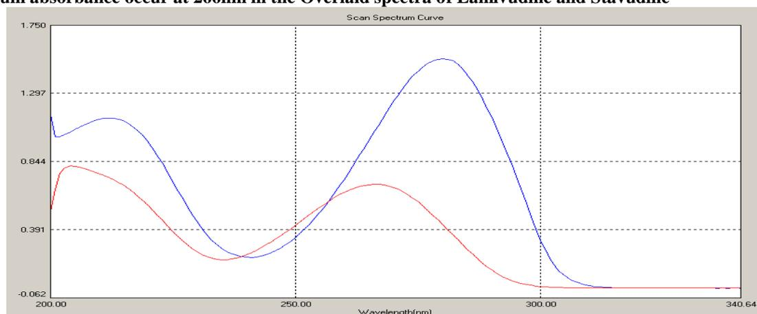
**Figure 1: UV maximum absorption spectrum of Lamivudine and Stavudine.**
