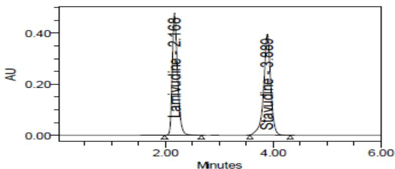
Figure 3: Chromatogram of accuracy 100% solution.
