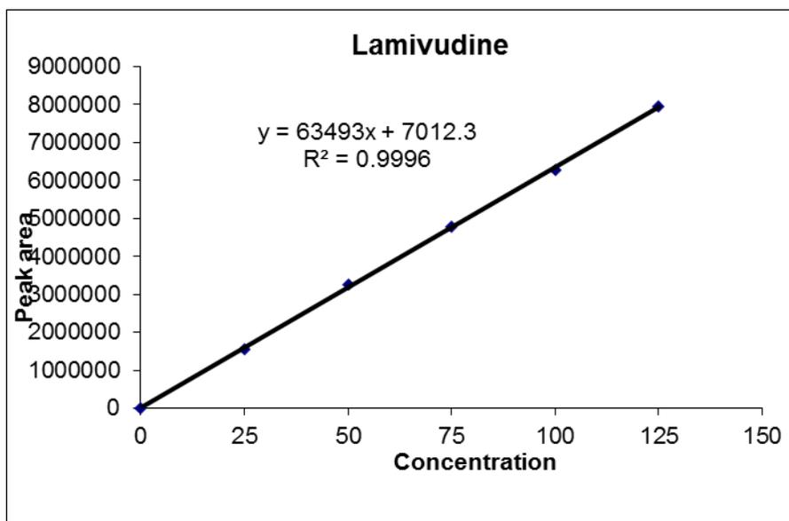
Figure 8: Chromatogram for linearity curve of Lamivudine.
