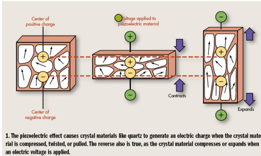
Figure 3: Piezoelectric effect.
