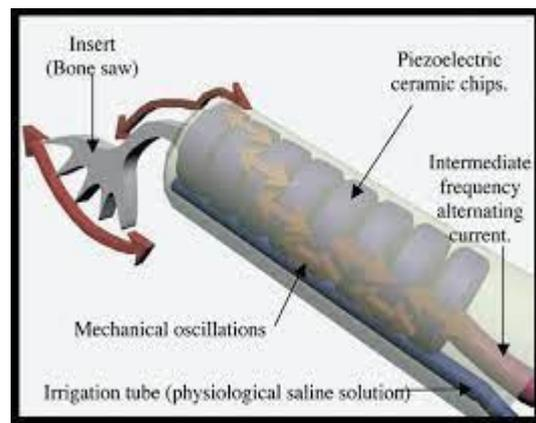
Figure 8: Irrigation tube, cutting saw.
