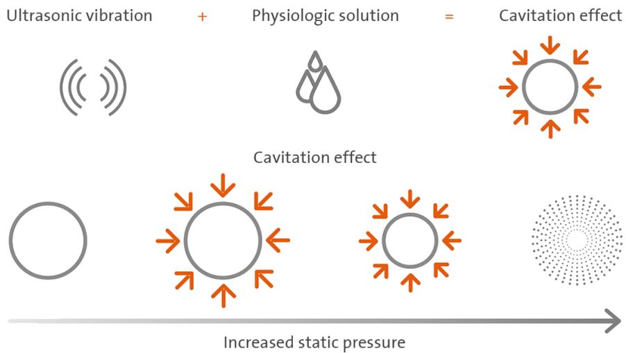
Figure 4: Cavitation Effect.
