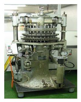
Common manufacturers of tablet presses include Fette, Korsch, Kikusui, Manesty and Courtoy. Tablet presses must allow the operator to adjust the position of the lower and upper punches accurately, so that the table weight, thickness and density can each be controlled. This is achieved using a series of cams, rollers, and/or tracks that act on the tablet tooling (punches).
