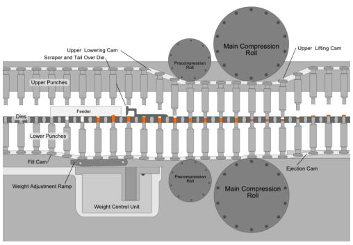
The tablet pressing operation: Tablet presses, also called tableting machines range from small, inexpensive bench-top models that make one tablet at a time (single-station presses), with only around a half-ton pressure, to large, computerized, industrial models (multi-station rotary presses) that can make hundreds of thousands to millions of tablets an hour with much greater pressure. The tablet press is an essential piece of machinery for any pharmaceutical and nutraceutical manufacturer.
