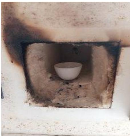
**Fig. 1: Acid soluble ash value determination.**
