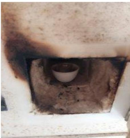
**Fig. 2: Water soluble ash value determination.**
