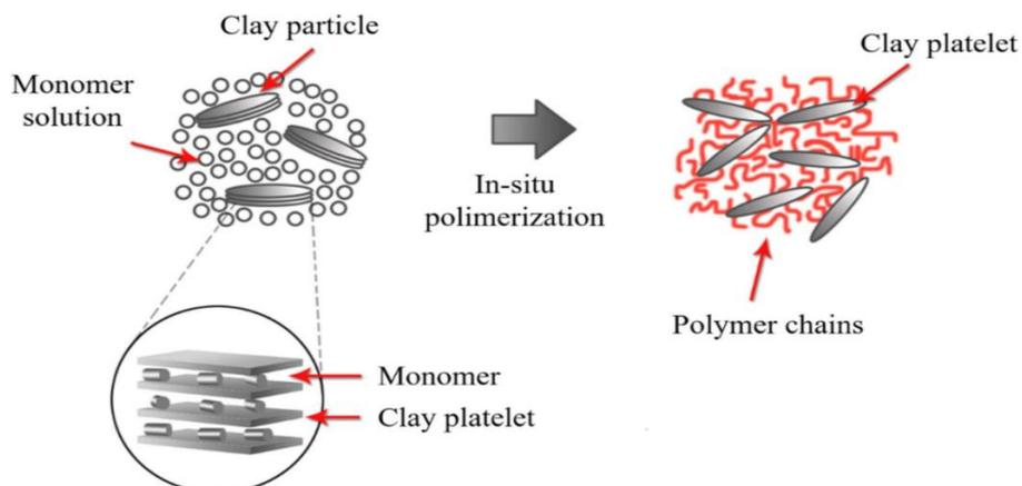
Figure No .14: Clay polymer nanocomposites.
