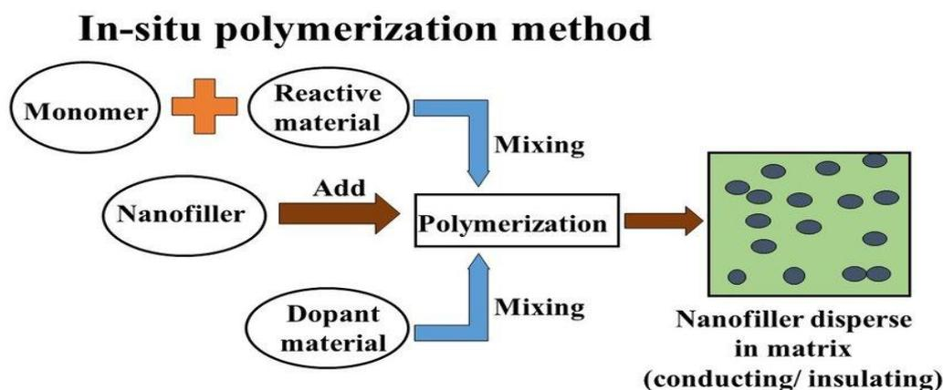
Figure No.6: In-situ polymerization method.
