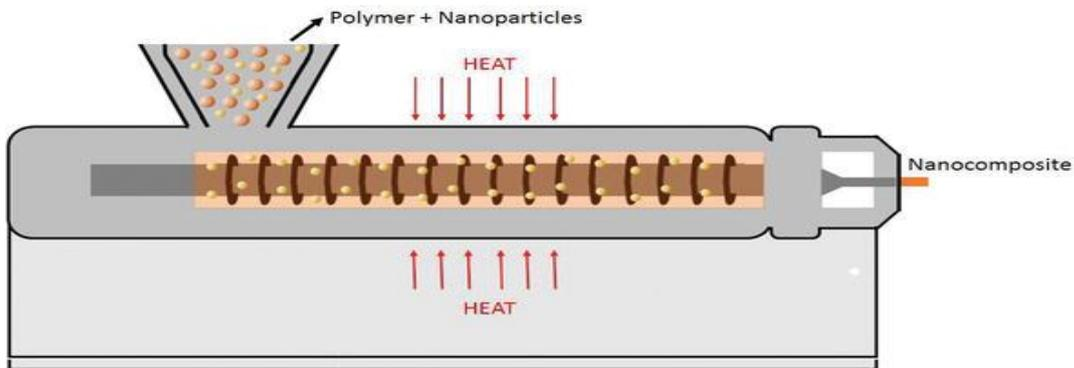
Figure No.9: melt extrusion method.
