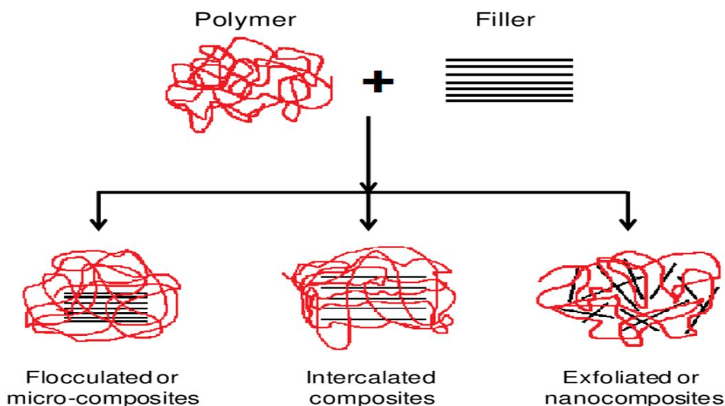
Figure No.5: Intercalated, flocculated and exfoliated polymer/layered silicates (clay) nanocomposites.
