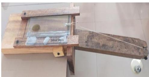
**Fig. 3: Apparatus showing Spreadability test for Phytosomal Cream and Gel.**
