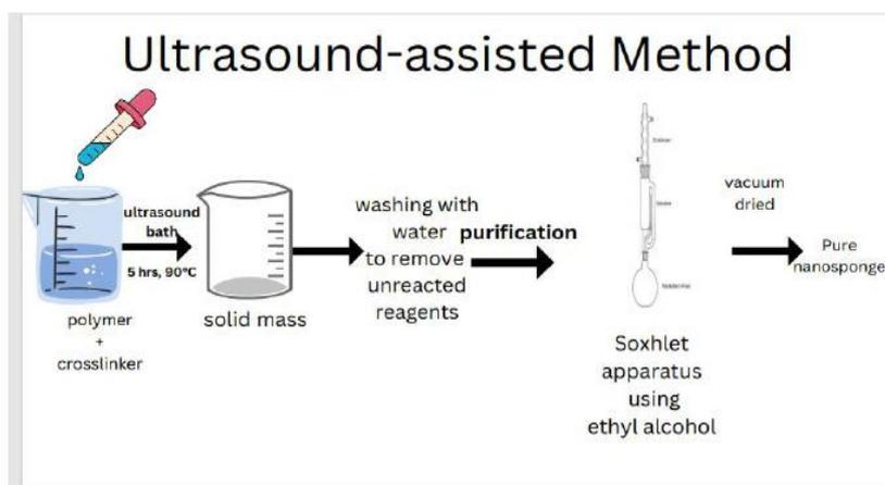
Fig. 7: Ultra sound assisted method.<sup>[6]</sup>
