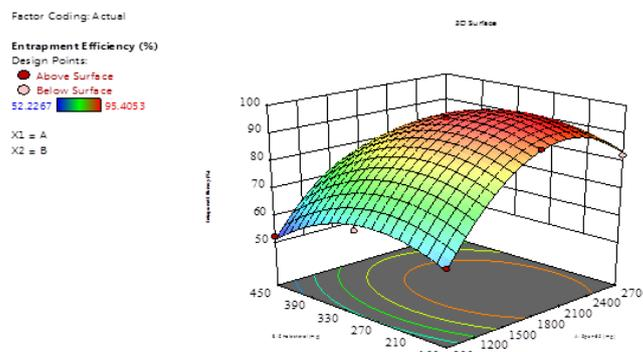
**Fig. 4: Response surface plots for the effect of amount of cholesterol and span 60 on % entrapment efficiency.**
