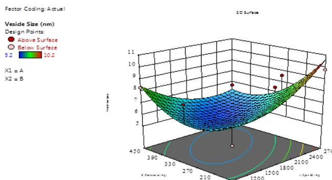
**Fig. 5: Response surface plot for the effect of amount of Cholesterol and Span 60 on particle size.**
