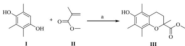
**Scheme 1: Synthetic pathway for Trolox methyl ester. (a) (HCHO)<sub>n</sub>, [CH<sub>3</sub>(CH<sub>2</sub>)<sub>3</sub>]<sub>2</sub>NH, CH<sub>3</sub>COOH, reflux, 20 h.**
