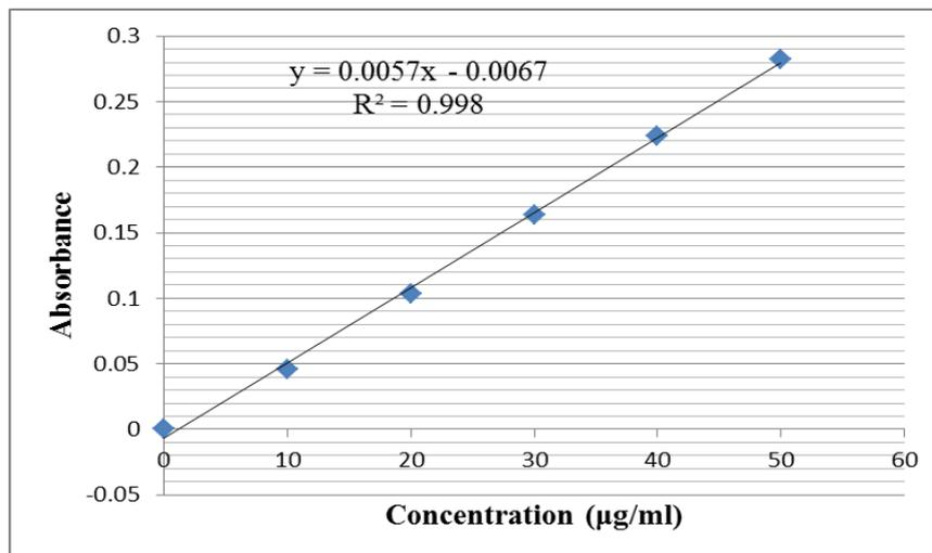
**Fig. 4. Calibration curve of Tenofovir disoproxil fumarate.****Accuracy**
